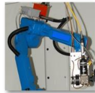
Figure 2: Robot material processing through the ultra-short pulse fibre delivery system.
