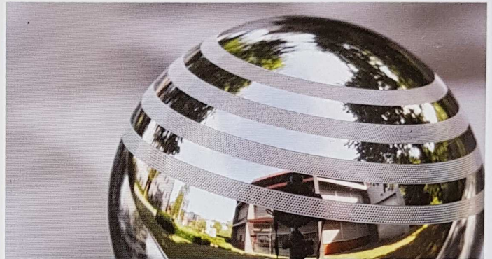
Different pillar patterns are applied in rings to this demonstrator.
