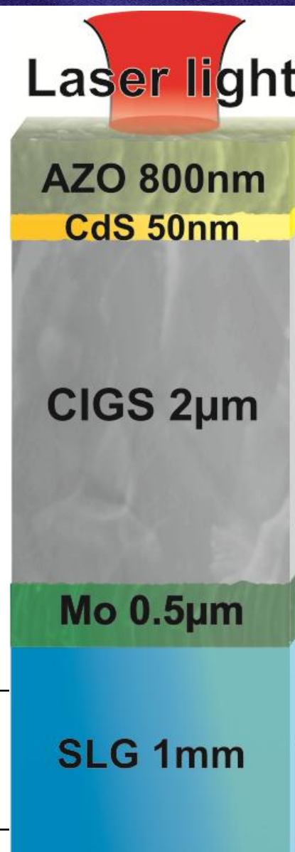
Fig. 2. Schematic cross-section of CIGS solar cell
