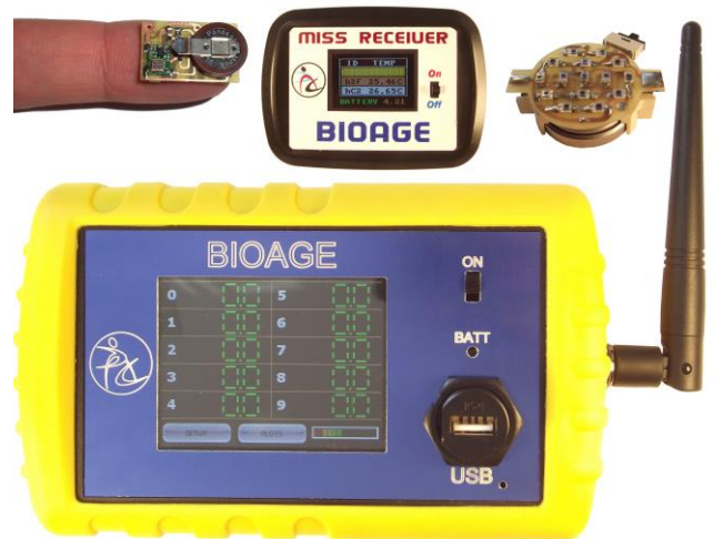
The smart microsensors and two hand-held data receiver; ©BIOAGE
